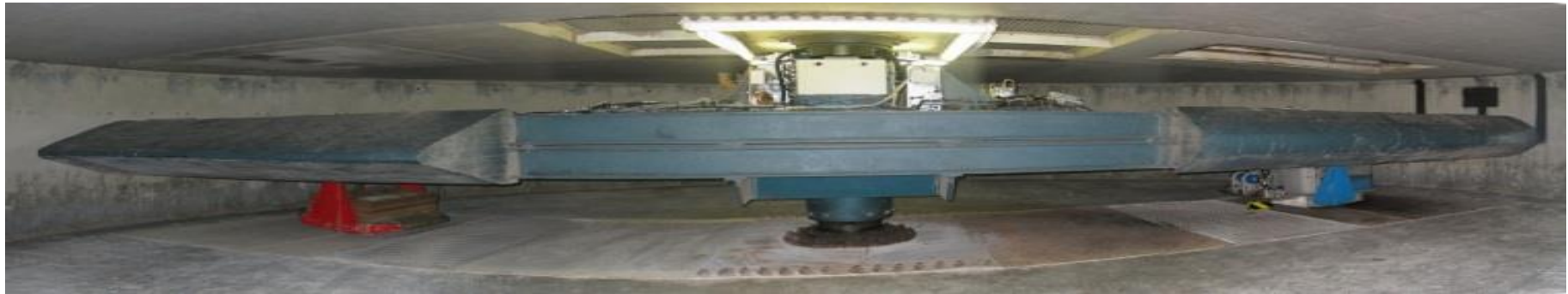
A view of the 10m diameter Turner Beam Centrifuge at University of Cambridge
